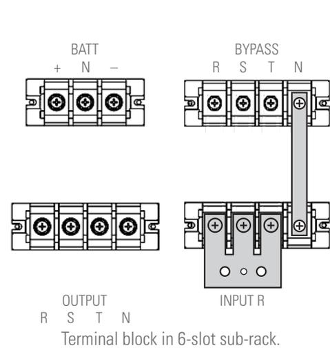
Terminal block in 6-slot sub-rack.
