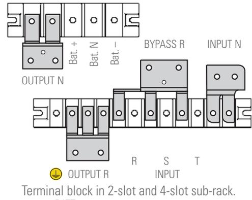
Terminal block in 2-slot and 4-slot sub-rack.
