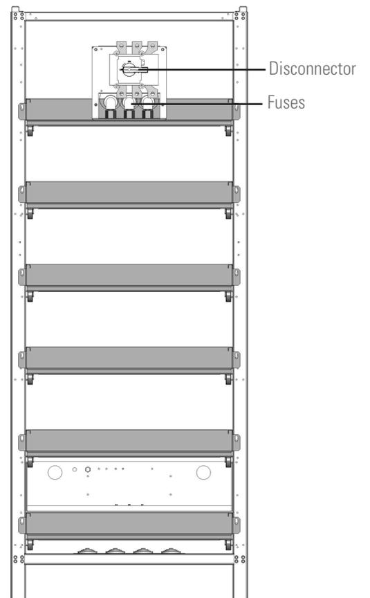
Fig. 9. Front view of battery cabinets.
