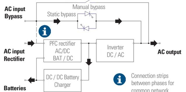
Fig. 20. Flowchart in Bypass mode.
