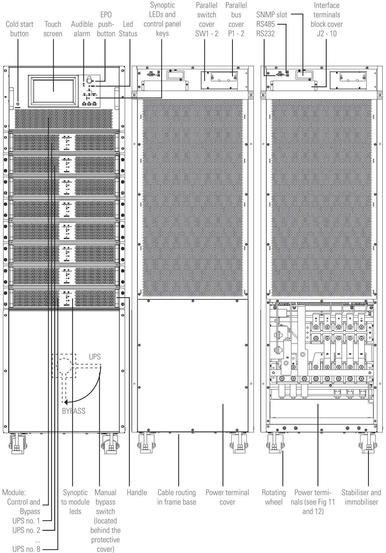
**i** The figure on the right shows the sub-rack with the terminal cover removed.
