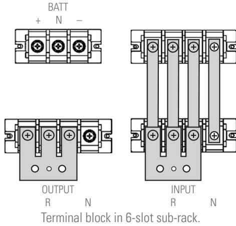
Terminal block in 6-slot sub-rack.
