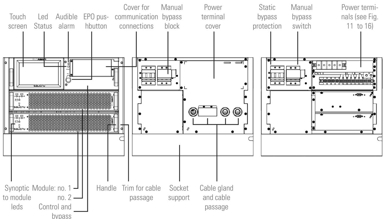
**i** When installing a sub-rack inside a cabinet, the static bypass and manual bypass switches on the back of the sub-rack will be inaccessible. In relation to the first one, it is necessary to set it to "On" before placing the sub-rack in the cabinet. The figure on the right shows the sub-rack with the terminal cover removed.
