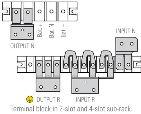
Terminal block in 2-slot and 4-slot sub-rack.
