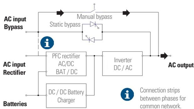
Fig. 21. Flowchart in manual bypass mode (maintenance bypass).
