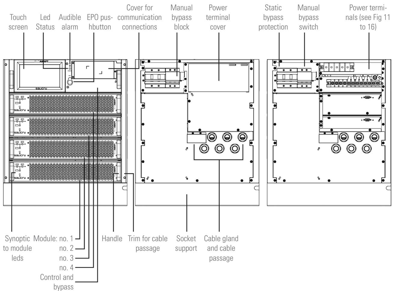
**i** When installing a sub-rack inside a cabinet, the static bypass and manual bypass switches on the back of the sub-rack will be inaccessible. In relation to the first one, it is necessary to set it to "On" before placing the sub-rack in the cabinet. The figure on the right shows the sub-rack with the terminal cover removed.
