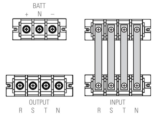
Terminal block in 6-slot sub-rack.
