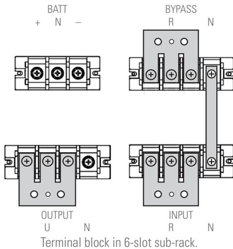
Terminal block in 6-slot sub-rack.
