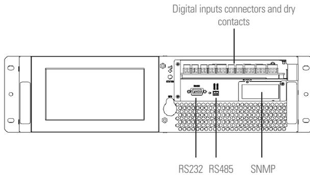
Fig. 37. Communication connections in 2 and 4-slot models.
