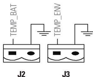
Fig. 39. Terminal block J2 and J3 for connection with sensors.
