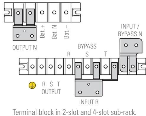
Terminal block in 2-slot and 4-slot sub-rack.
