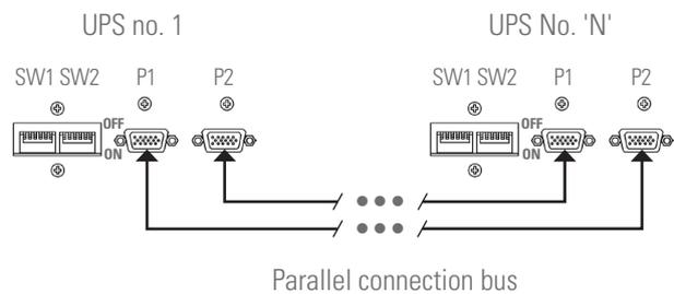
Fig. 33. DB15 connectors on the communication bus.
