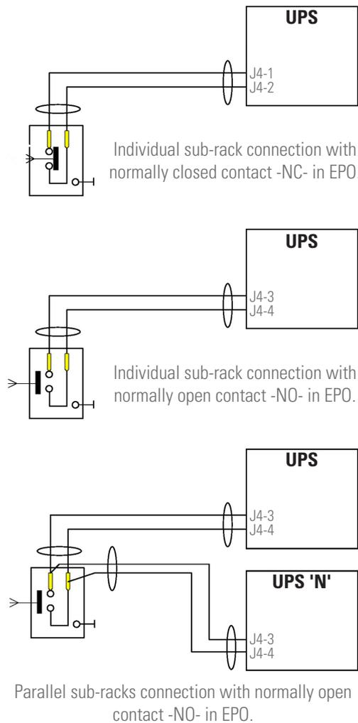
Fig. 41. External EPO connection with device or devices.
