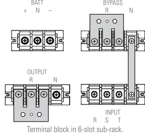
Terminal block in 6-slot sub-rack.
