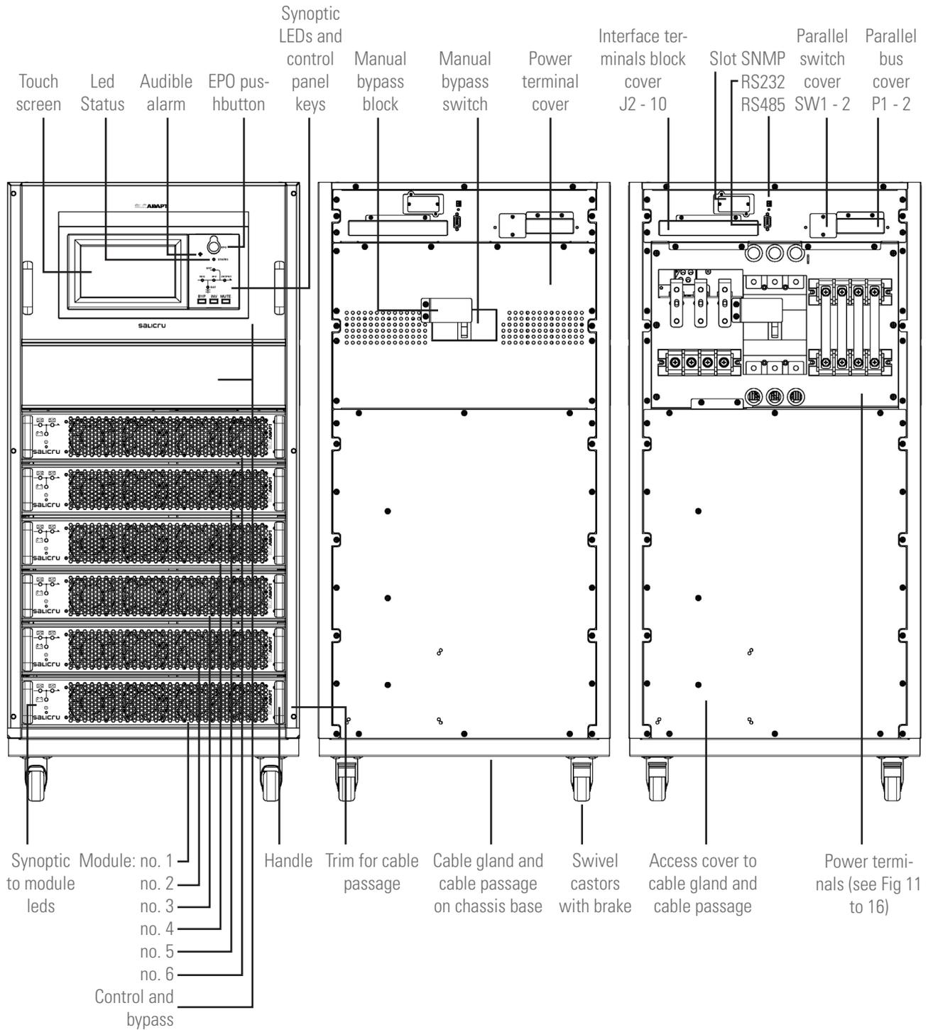
**i** The figure on the right shows the sub-rack with the terminal cover removed.
