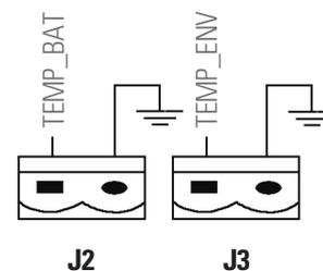
Fig. 66. Terminal block J2 and J3 for connection with sensors.
