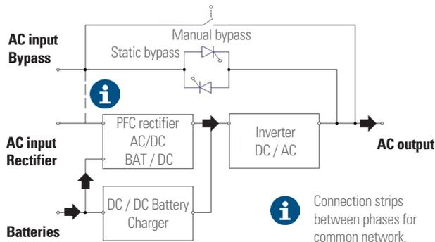
Fig. 19. Flowchart in Battery Mode.
