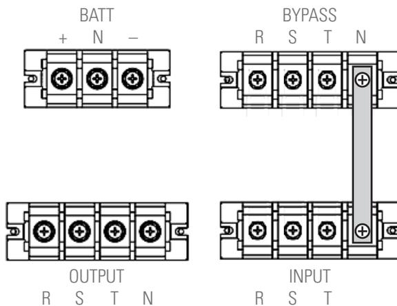
Terminal block in 6-slot sub-rack.
