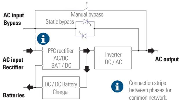
Fig. 18. Flowchart in Normal Mode.
