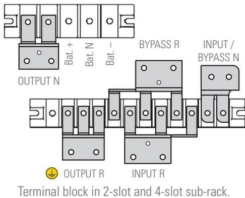
Terminal block in 2-slot and 4-slot sub-rack.
