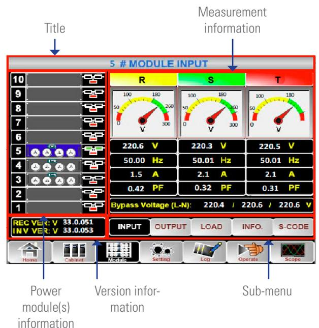
Fig. 54. Information menu of the module or power modules. Main sub-menu.
