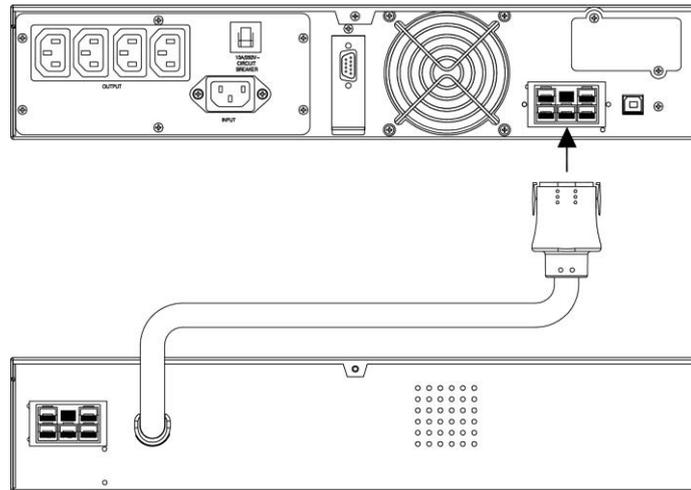
Example of connecting to external battery pack
