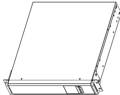
The demonstrations of UPS tighten up with rack mounting ears.
