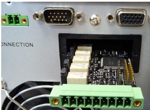
Fig. 8. Inserting the NIMBUS AS400 card
