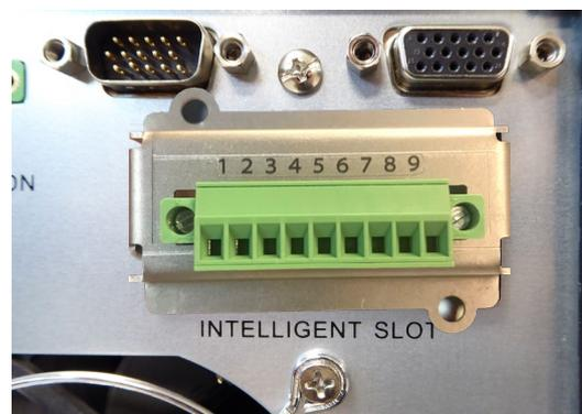
Fig. 11. Exclusive connector for SLC TWIN PRO2 0 - 3 kVA series.
